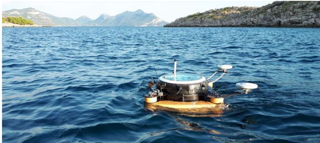
Autonomous USV for water sampling and surface surveying.
